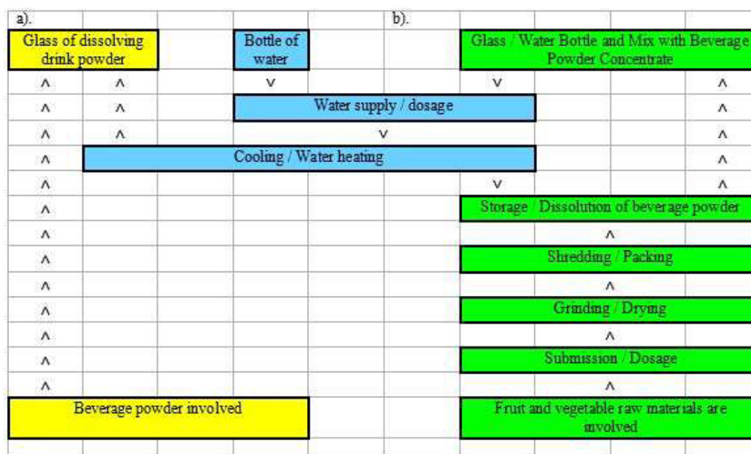
Fig. 3 Schematic diagram of structural and technological layout of coolers of a wide range of finished products: a – existing desktop; b – modernized floor
