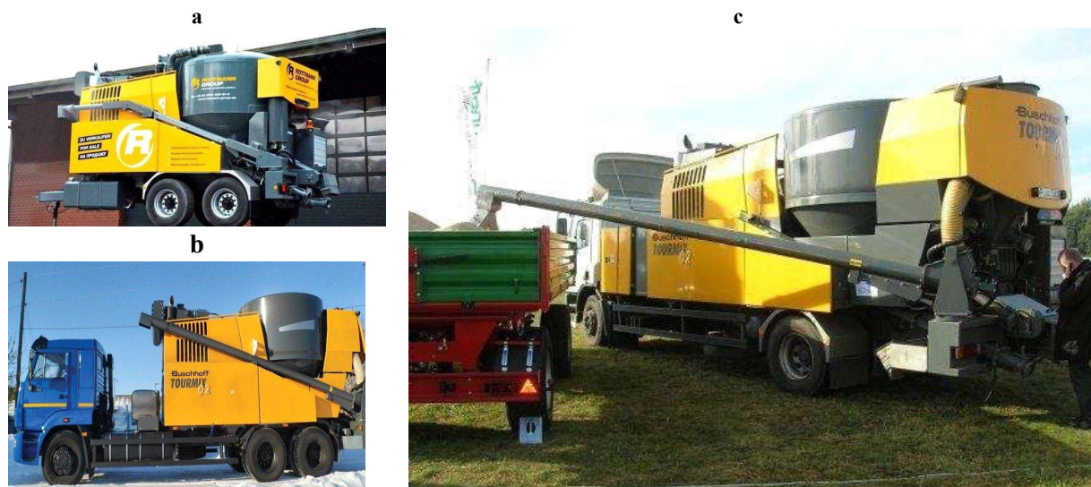
Fig. 4 Appearance of a mobile mini complex of production and distribution of compound feed trailed to a tractor or car (a), self-propelled on a car chassis (b) and in combination with various additional vehicles (c)
