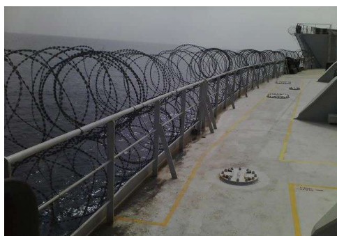
Fig. 8. The barbed wire application of the Stile Rocher ship
