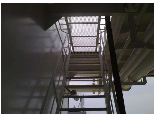
Fig. 9. Wire barrier application that can be opened on one side of the Stile Rocher ship
