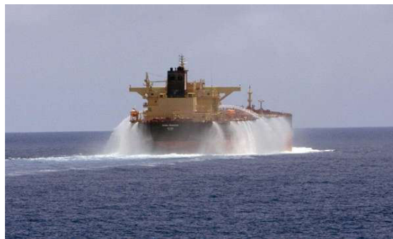
Fig. 7. Pressurized water application with fire hoses at pirate zone crossings on a commercial ship
