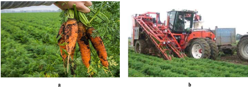
Fig. 3. The body and a fairly thick cover layer of carrots contain many nutrients (a. [11]), but insufficient mechanical strength with existing means of mechanized harvesting (b. [12])
