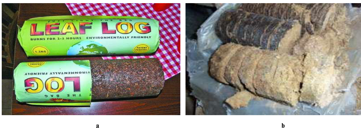
Fig. 3. General view of typical fuel briquettes from fallen leaves, where the binding material is 30% wax (a) [10] and 20% lignin (b) [11]
